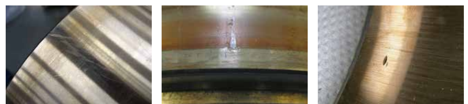
Indentation by handling When bearing surfaces are dented or gouged by hard, sharp objects.
