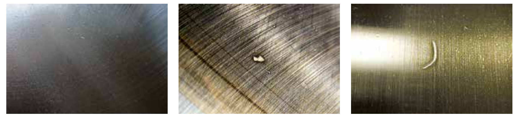
Indentation from debris When particles are over-rolled.
