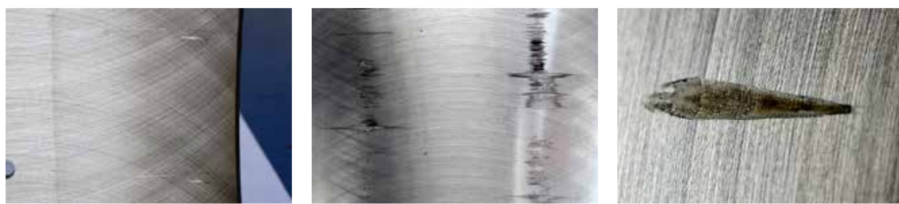
Adhesive wear A transfer of material from one surface to another.
