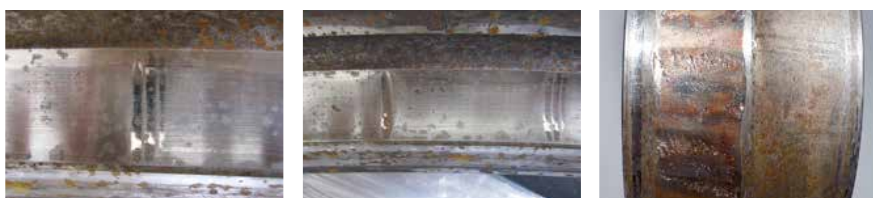
Frictional corrosion – False brinelling A formation of shallow depressions resulting from micro-movements under cyclic vibrations.
