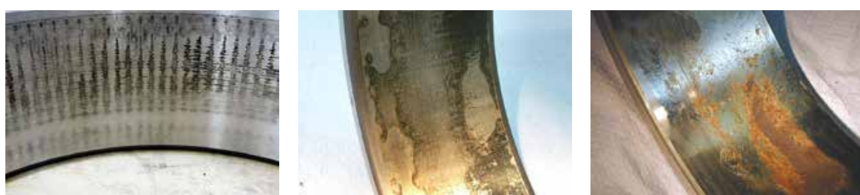
Frictional corrosion – Fretting corrosion The oxidation and wear of surface asperities under oscillating micro-movements.
