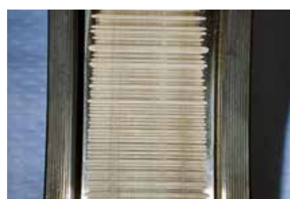
Current leakage The generation of shallow craters that develop into flutes that are equally spaced.
