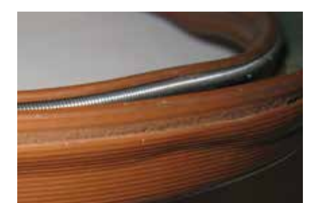
Seal damage Seal outside diameter damage due to poor lead-in chamfer and/or incorrect installation methods.
