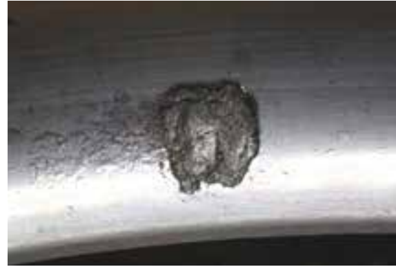
Subsurface initiated fatigue The initiation of micro-cracks at a certain depth under the surface.
