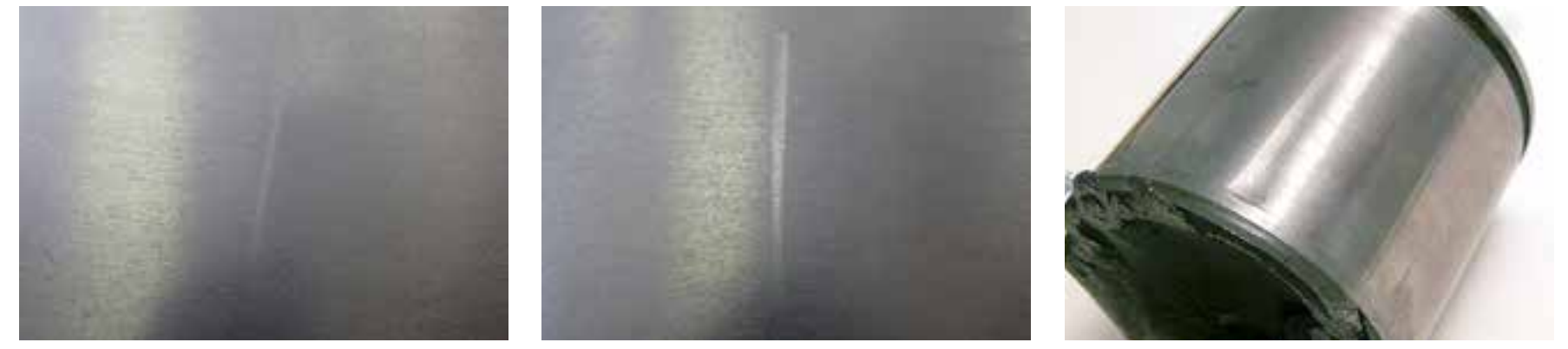
Overload The formation of shallow depressions or flutes in the raceways.
