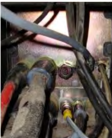
5 pin cable attached to feed-thru
